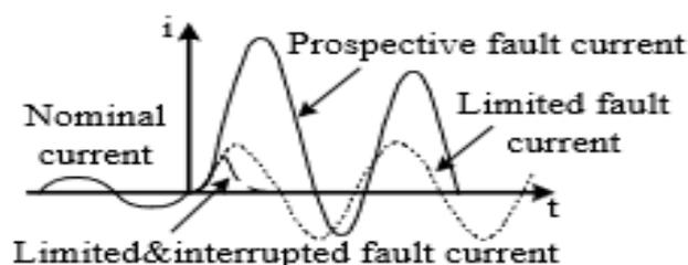
**Figure 1:** Typical waveform of a fault current with and without an FCL.
