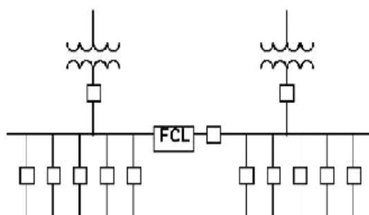
**Figure 5:** Fault current limiter in the bus tie position. The two buses are tied, yet a faulted bus receives the full fault current of only one transformer.
